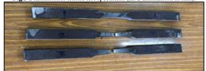
Fig.4 Tensile test specimens after a fracture.
