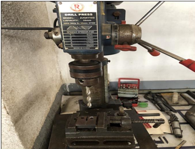
Fig.10 Using the drill press to have the hole compact tension CT specimen.
