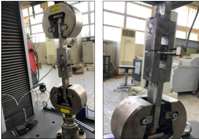
Fig.20 Tensile Test Machine and Test setup for CT type specimen.
