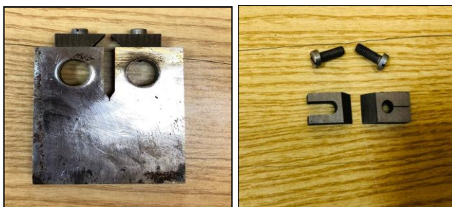
Fig.16 Attachable knife-edge design.
